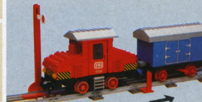
Automatic shunting. A trip post flicks the switch from forward to reverse.
